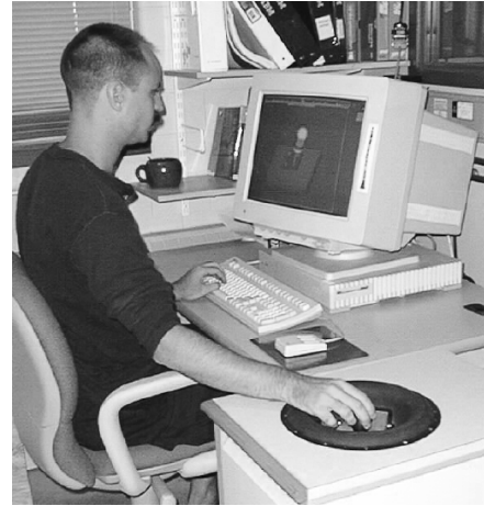
Figure 3: Using the Haptic Interface Device with a Graphics Display
