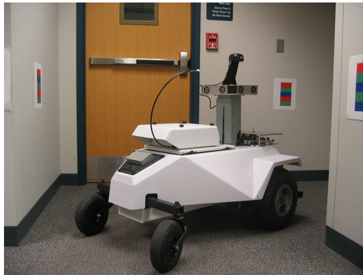
Figure 6.9: ‘LAGR’ robot navigating a corridor. Three color-coded landmarks, which are used by the vision based localization system, are visible in the image.
