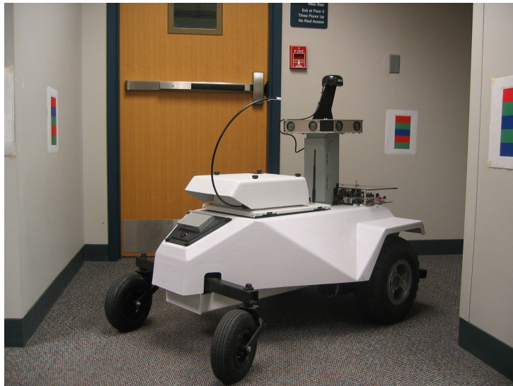
Figure F.4: The LAGR robot uses four stereo cameras to perform vision based localization while navigating. Three color-coded landmarks, which are used by the vision based localization system, are visible in the image.
