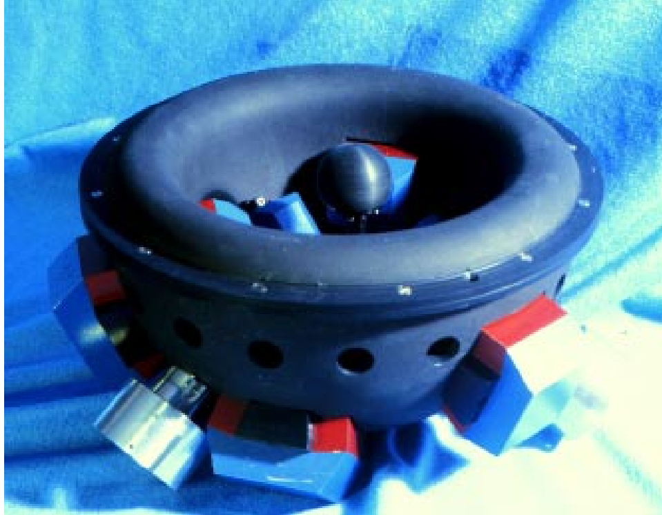
Figure 6.2: New Fabricated Lorentz Levitation Haptic Device
