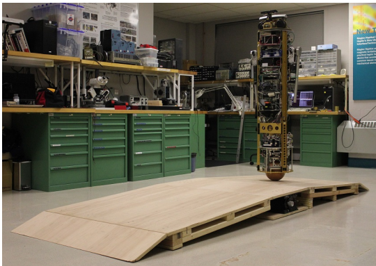
Fig. 6: The ballbot station-keeping on a variable-slope ramp.
