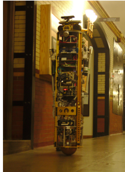
Fig. 1: The ballbot, a dynamically balancing mobile robot, operating on a sloped surface.
