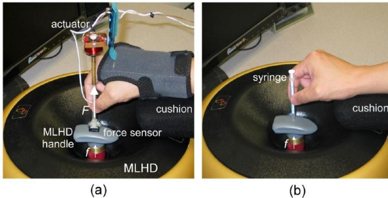
Figure 2. Illustration of the experimental setup. The user's perception of force was compared across the magnifier-ON/OFF conditions (a) and control condition (b). A magnetic levitation haptic device (MLHD) was used to produce the experimental stimuli.
