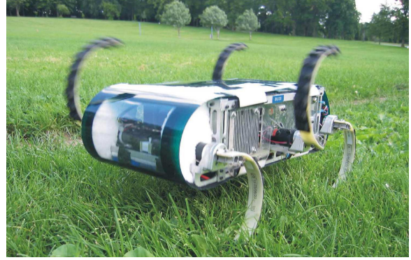
Fig. 2. RHex running outdoors on a grassy surface in a standard tripod gait.
