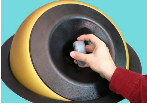
Fig. 3. New second-generation 6-DOF magnetic levitation haptic device: overall view showing the spherical swivel mounting in a desktop which allows re-orientation to suit users' preferences
